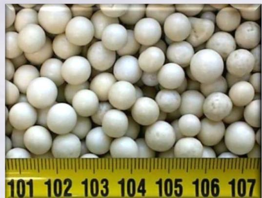
*Pellets produced with MemPhos® pellet reactor
