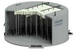
in the downstream aerobic treatment. Thanks to Colsen's carefully designed distribution system, the wastewater is divided evenly over the surface. The dense granular sludge bed ensures a compact reactor thanks to the Colsen designed three phase separators.
