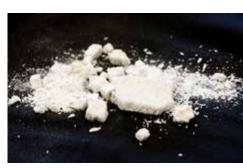
Secondly, magnesium is dosed in a reaction tank. Magnesium reacts with the present phosphorus (as phosphate) and ammonium forming struvite. After this precipitation phase, struvite is settled, discharged and dewatered. The formed product is readily accessible as substitute for agricultural fertilizers or as a phosphate ore.
